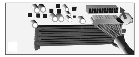
4. Connect the 8-pin or 4+4-pin connector for the CPU. If your motherboard has an 8-pin socket with a cover on some of the openings, we recommend that you remove the cover and use the 8-pin connector.
